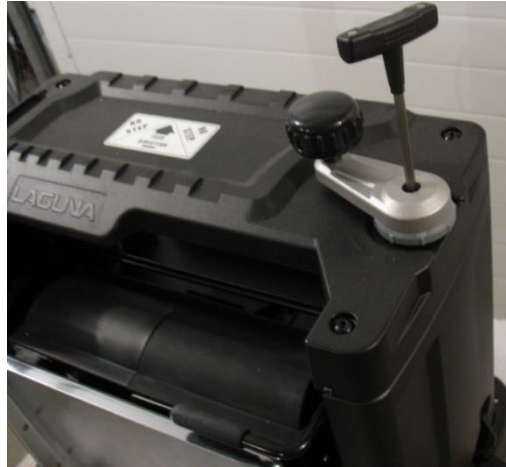
Figure 3: Installing Thickness Adjustment Handle
