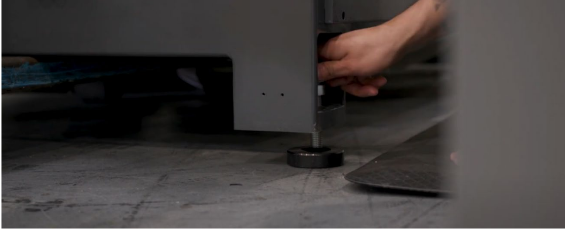
Figure 8-2: Aligning the Metal Feet
