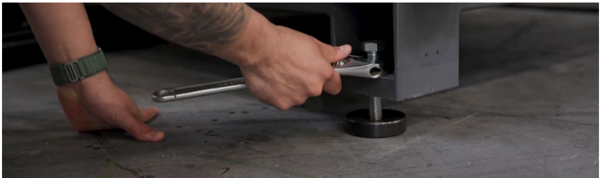
Figure 8-3: Using a Crescent Wrench to Adjust and Tighten the Bolt/Nut Combo
