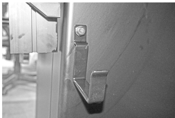
Fence Hook Installation
