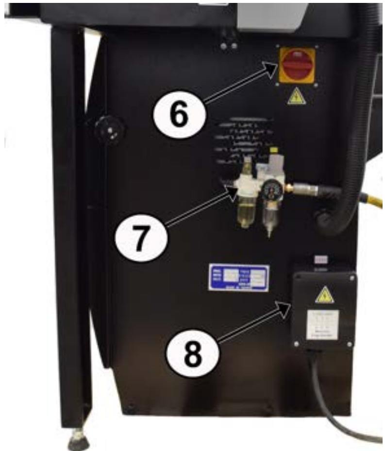
Figure 3–1: Power and Air Fence
