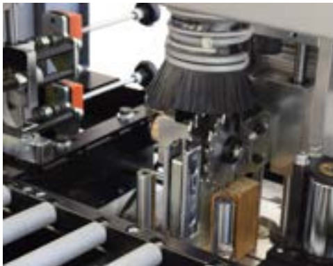
Figure 10-10: End Trimmer Raised with Wood Block
