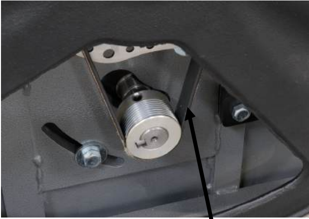
Motor drive pulley Drive belt
