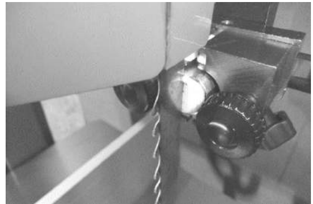
Back guide touching the back of the blade
