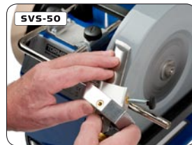
Multi Jig For skewes of any shape, even with an oval section.
